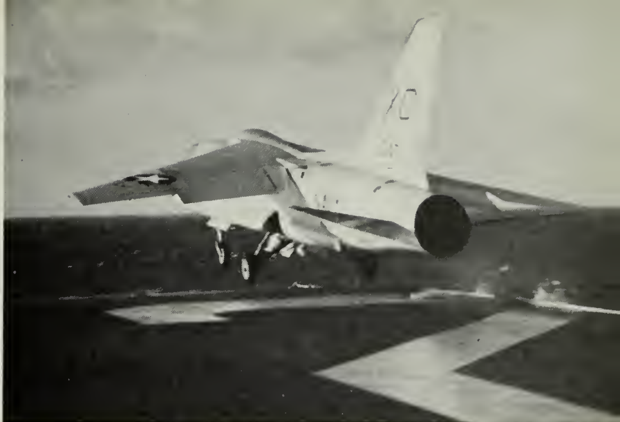
OFF WE GO—Steam catapult blasts pilot and plane skyward with a mighty roar as an F8U-1 Crusader takes to the air on a morning mission at sea.
